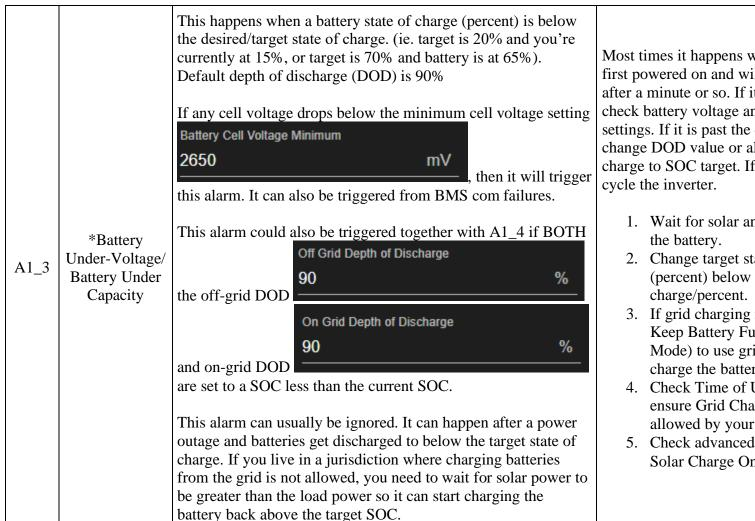
Most times it happens when an inverter is first powered on and will clear on its own after a minute or so. If it does not, double check battery voltage and depth of discharge settings. If it is past the depth of discharge, change DOD value or allow batteries to charge to SOC target. If all else fails, power
