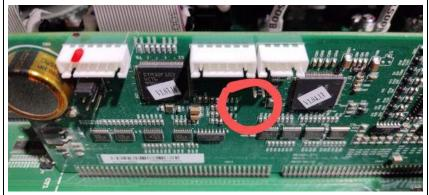
When these terminals are connected, the inverter makes measurements on the grid and load terminals to make sure there is no voltage before proceeding with the test mode. If there is voltage, it triggers this fault so that the inverter is not damaged by external power during the test.
